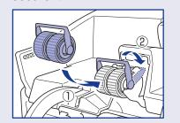
4. Push the lock lever for the feed roller down (①) and to the right (②).
