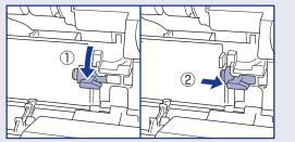
5. Align the notches in the shaft of the feed roller with the pins on the s scanner, and place the feed roller into position.
