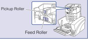
Be sure to install the pickup roller and feed roller, as documents will rollers are not installed.
